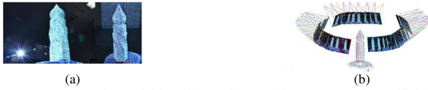
Figure 1. (a) photogrammetric acquisition of the white test object “Testy” using artificial texture from 3 video projectors. (b) result of orientations and sparse point cloud for 46 images. (Wenzel et al., 2013)
